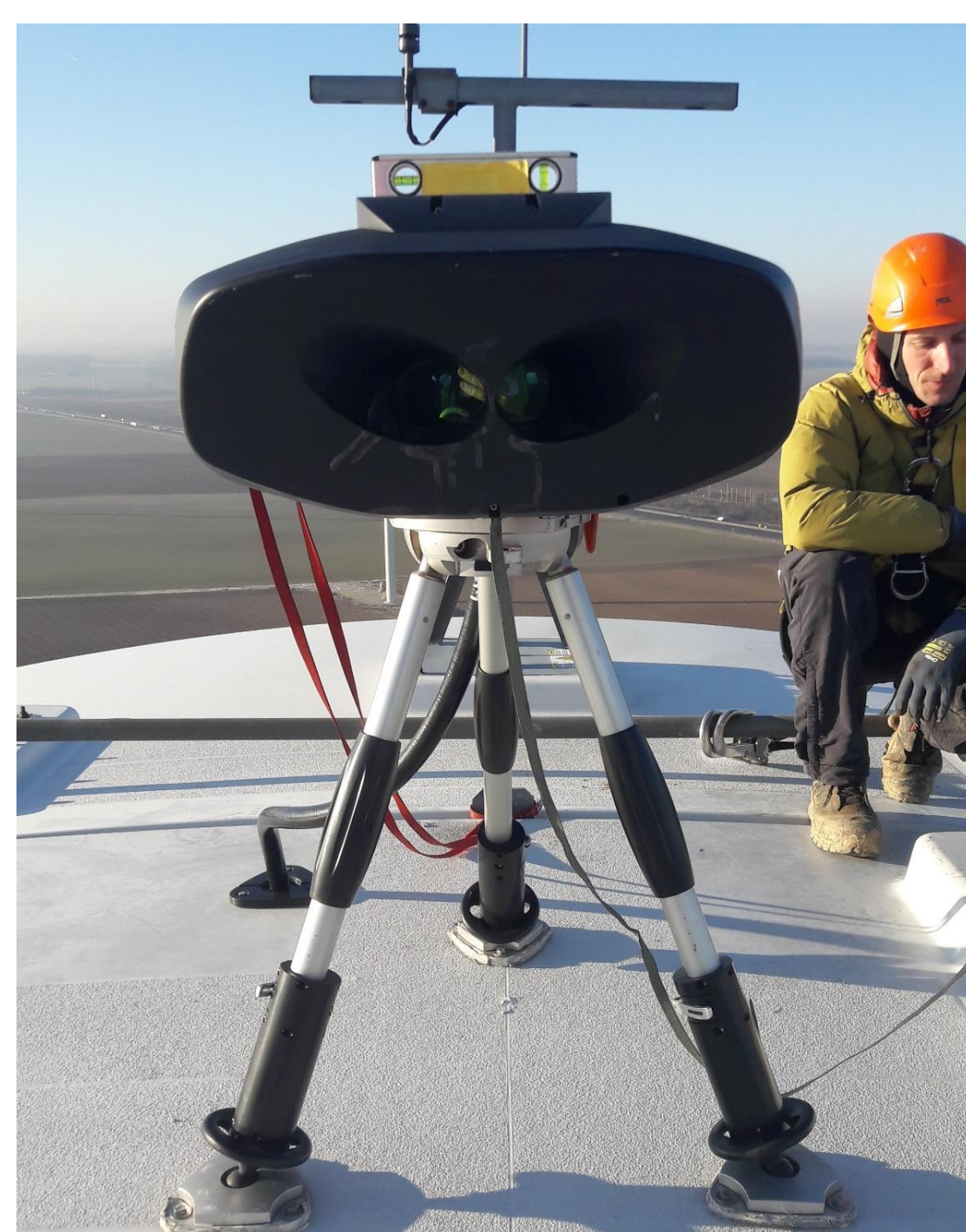
Wind Iris measuring from 80 to 400 m distance
